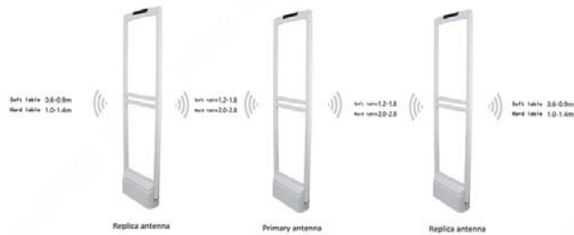
Figure 3-12 One primary and two replica antennas
